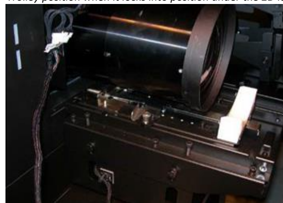
Trolley position when it locks into position under the 2D lens
